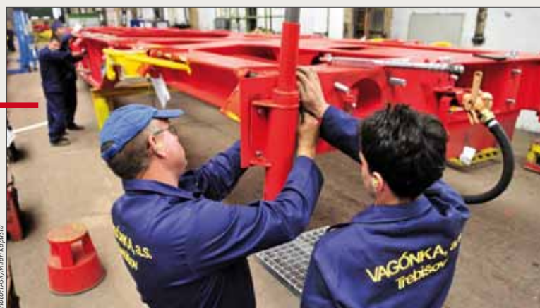
Installation of new prototype of Sggmrss 90 container goods wagon by Tatravagónka Poprad – Vagónka, a.s. Trebišov.
