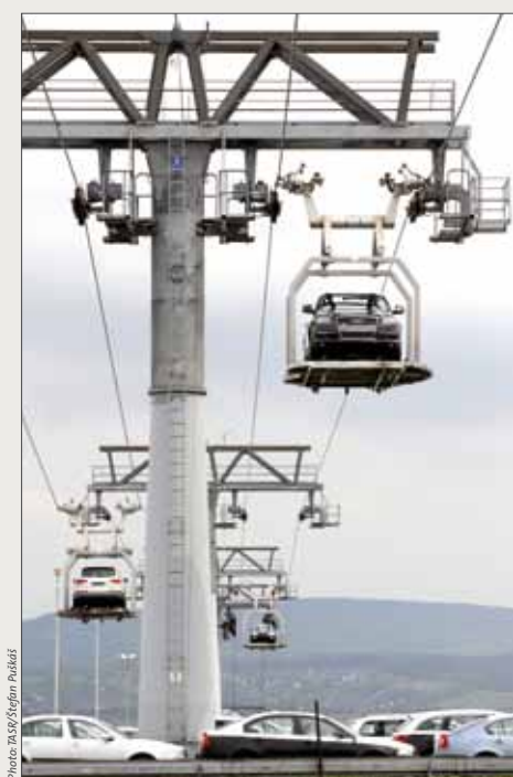
An unique arial car transportation via cableway to a trial polygon, Volkswagen plant, Bratislava.
